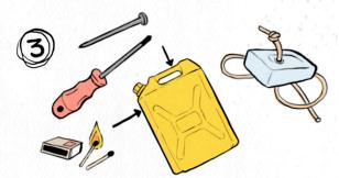
USE A SHARP TOOL TO PIERCE Q HOLES INTO THE JERRY CAN - ONE AT THE TOP INTO THE HANDLE AND ONE AT THE FRONT. HEAT UP THE TOOLS TO HELP MELT THE PLASTIC OF THE JERRY CAN. PIERCE A HOLE INTO THE SOAP TO ATTACH A STRING. FILL THE JERRY CAN WITH WATER AND CLOSE IT WITH A CAP.
